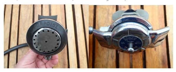
While the intrepid trio were at it, they decided on punching a hole through the front cover plate, big enough to put a finger through & operate the diaphragm/fulcrum lever to get a free-flow, when needed. The obvious more elegant solution came next. A rubber knob, glued to the diaphragm & protruding through the cover plate. History does not record, whether that was inspired by someone's pinkie getting stuck!
