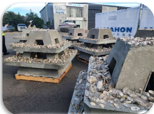
The concrete modules at McMahon's Port Adelaide dockyard prior to sinking.
